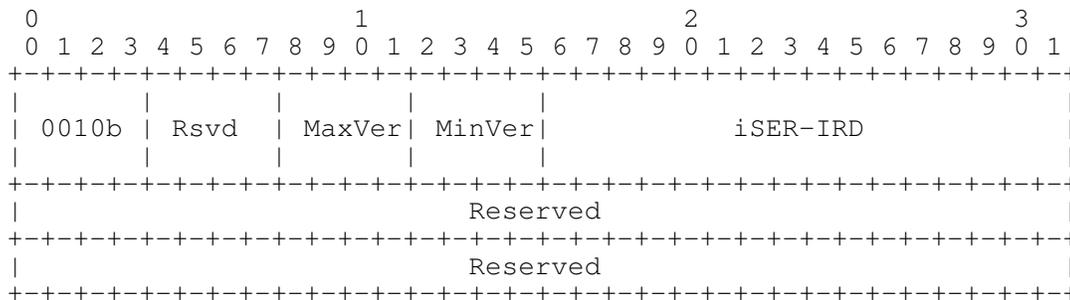
Figure 4 iSER Header Format for iSER Hello Message
