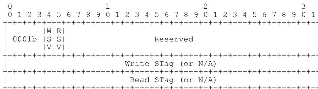
Figure 3 iSER Header Format for iSCSI Control-Type PDU
