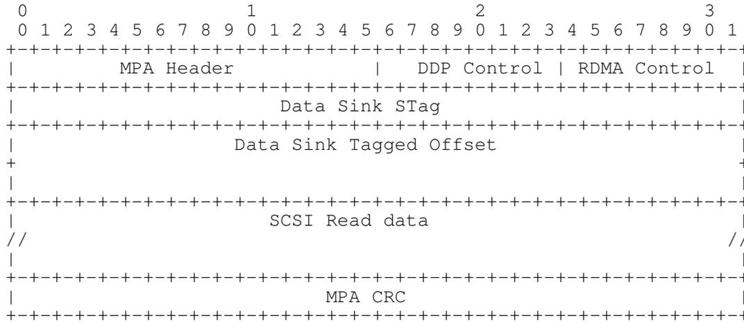
Figure 9 RDMA Write Message containing SCSI Read Data
