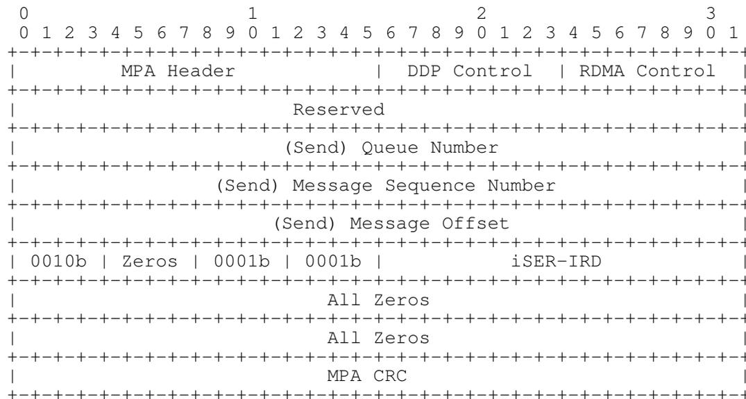
Figure 6 SendSE Message containing an iSER Hello Message
