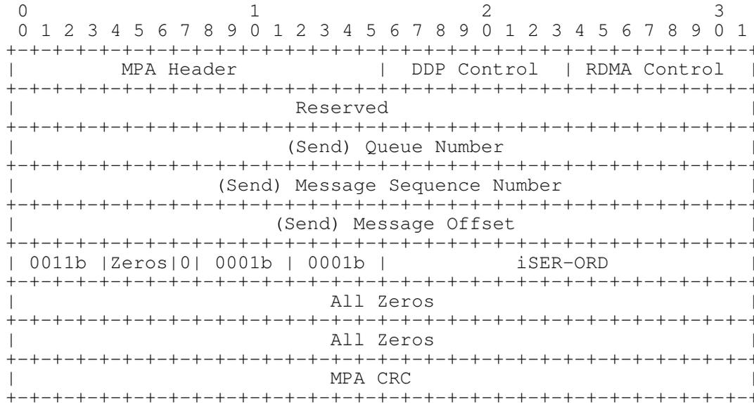
Figure 7 SendSE Message containing an iSER HelloReply Message
