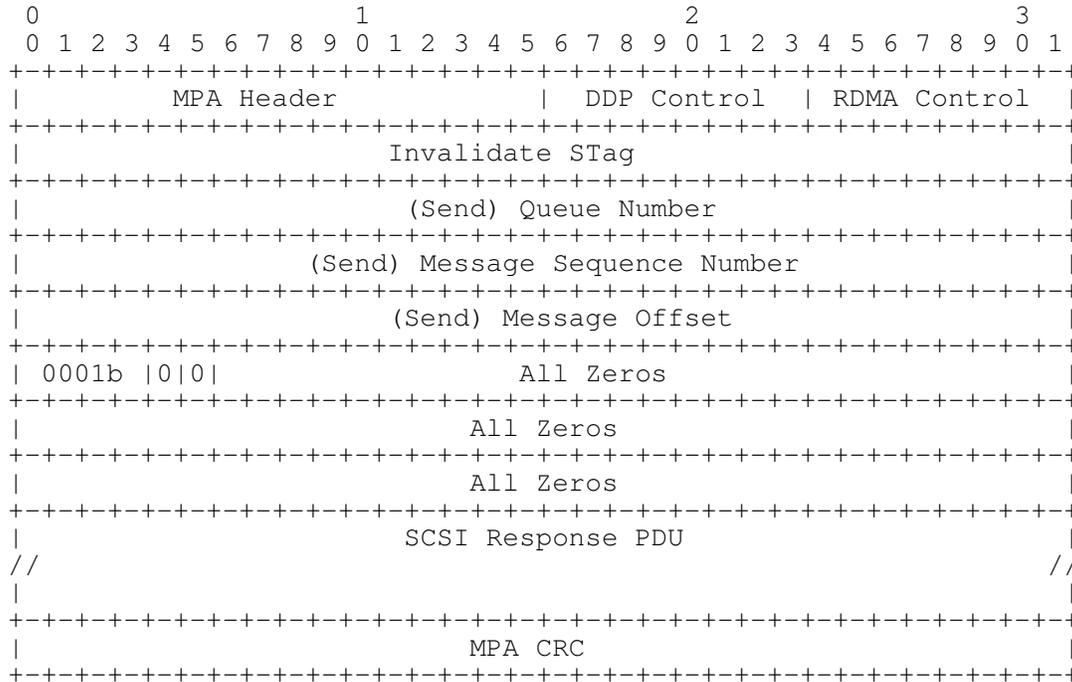
Figure 13 SendInvSE Message containing SCSI Response PDU
