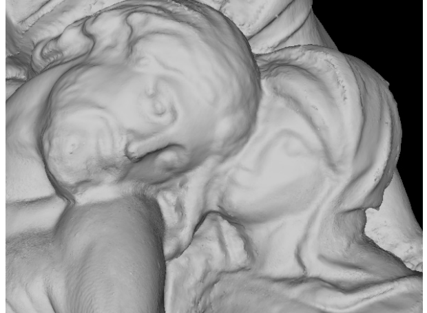
Fig. 1. Section of Michelangelo’s Florentine Pietà. This 14M triangle mesh was generated from more than 700 scans using the ball pivoting algorithm.
