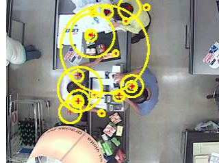
Figure 2. STIPs detected in one frame. Each STIP (circle) is associated with a location (center), spatial scale (radius) and temporal scale (not shown here). Several STIPs are detected near the hands of the cashier, but many are caused by the bagging person and the customer.
