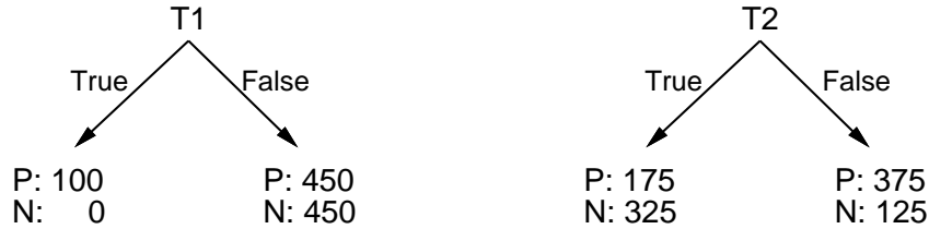
Figure 3: A numerical example illustrating how standard test selection functions can overlook nuggets. Both the Gini Index and the information gain function prefer T2 over T1, whereas our selection function prefers T1.
