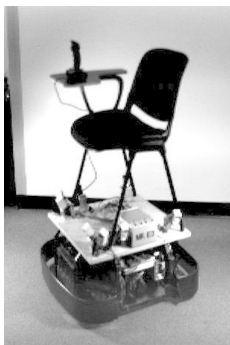
Figure 1. Our mobile robot has a seat for a passenger. To steer the vehicle the driver can directly interact with the navigation sensors, make suggestions through the joystick, or authorize various activities using a bank of toggle switches.
