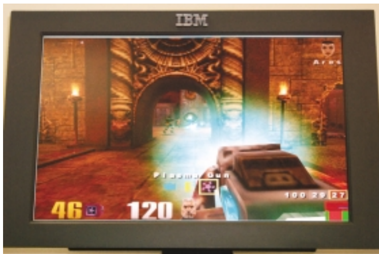
5 Using the Chromium software, we can play Quake III Arena at a resolution of 3840 \times 2400 pixels.
