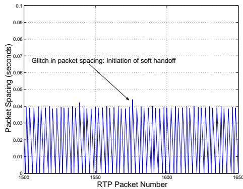
Figure 13. Spacing between the RTP packets
