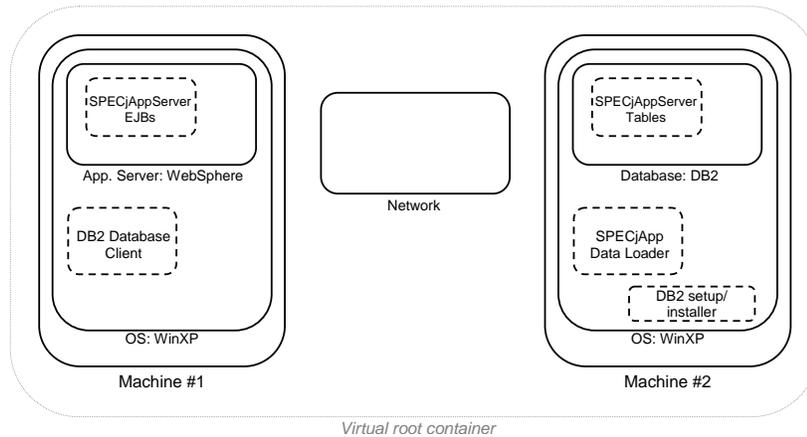
**Figure 1: SPECjAppServer scenario.** The figure shows the SPECjAppServer configuration scenario represented in our abstract system model of nested containers and configuration controls. Containers with solid lines are hosting environments; those with dashed lines represent system resources.
