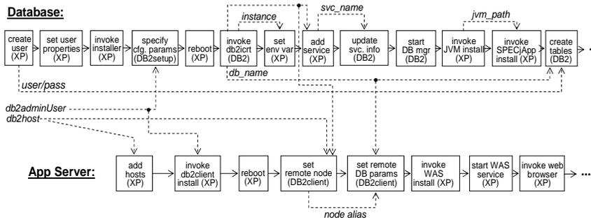
**Figure 2: Partial manual configuration procedure and action sequence for SPECjAppServer scenario.** This figure shows part of a manual configuration procedure for installing SPECjAppServer on a two-machine system using IBM’s WebSphere Application Server v5.1 and DB2 Universal Database v8.1. Each box represents a configuration action, and the dotted arrows represent the flow of configuration parameters between actions. Each action applies to a specific container, indicated in parentheses.
