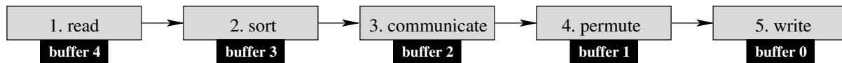
Figure 1: An implementation of out-of-core column sort, represented as a pipeline. The first stage reads data from disk into a buffer. The second stage performs a local sort. The third stage performs interprocessor communication. The fourth stage performs a local permutation. The final stage writes data from the buffer to disk. The stages run concurrently so that, at any moment, each stage may be working on a distinct buffer.
