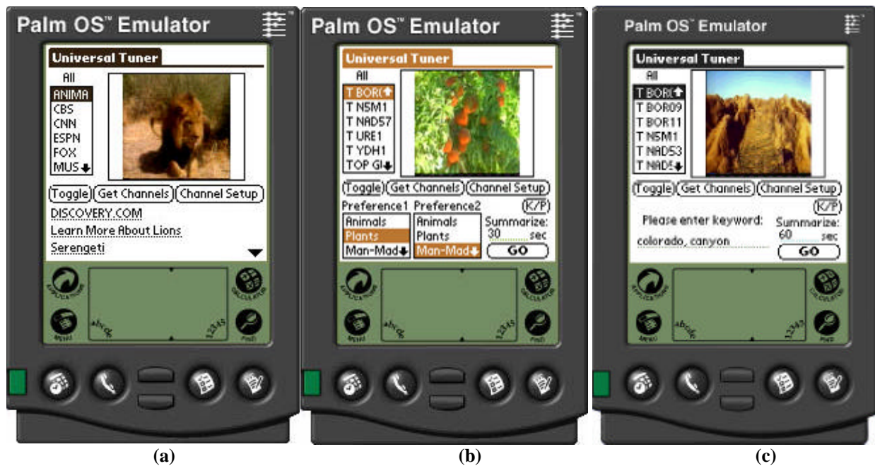
Figure 2: The User Client Interface on the Palm OS PDA for 3 Personalized Video Scenarios: (a) Video-on-demand with interactive hyperlinks, (b) Summarized video based on preference topics and time constraint, and (c) Summarized video based on query keywords and time constraint.
