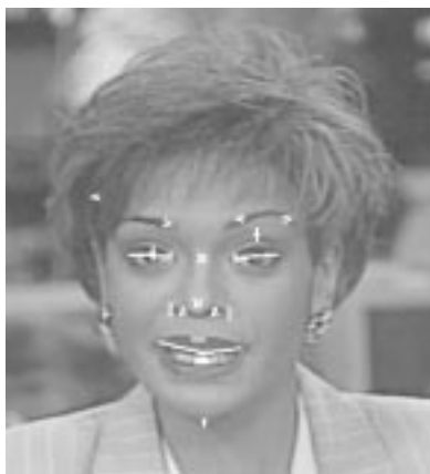
Figure 1. A diagram of a face showing, in white, the automatically located features.
